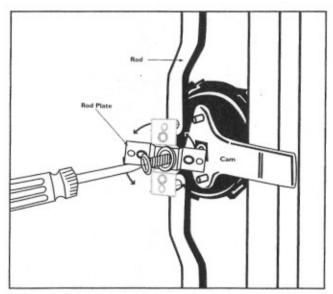
Loosen screw and rotate rod plate on back of handle. Place rods through holes at top and bottom of door and then attach to cam. Rotate rod plate back to its original position and re-tighten screw to secure rods to door handle.
